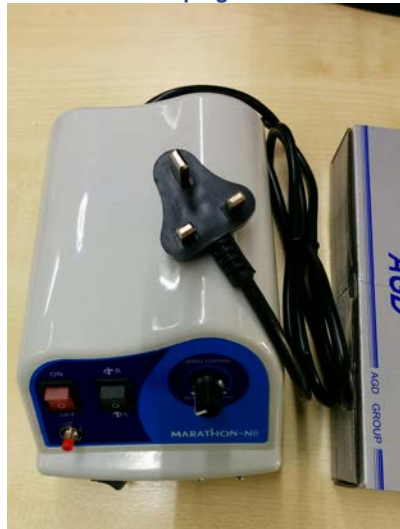
Unsafe electrical plug
